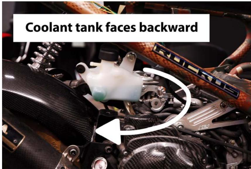
3. Relocate any tubing (fuel and PCV) and any wiring that is located above the square frame cross brace and move it below this brace. Zip-tie things down and make sure nothing binds when the engine pivots.
